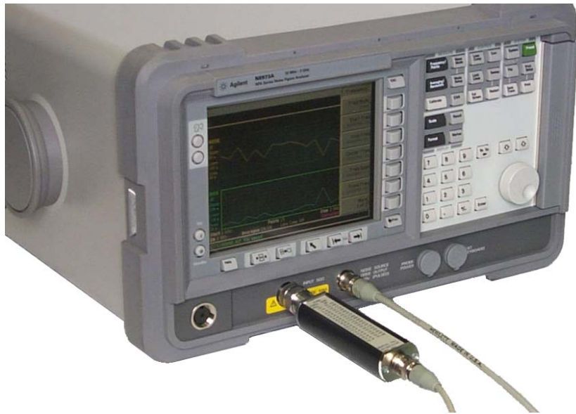
Figure 1-1 NFA with a Normal Noise Source connected
