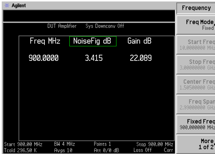
Figure 1-7 Typical Fixed Frequency Measurement Result in Meter Format.
